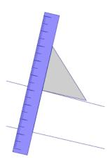
Slide the setsquare along the ruler. Try to line up with the other line. If the edge of the setsquare aligns with the line, the two lines are parallel. If the edge of the setsquare does not align with the line, then the two lines are not parallel.
