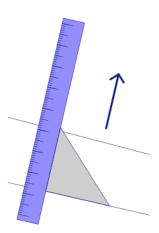
Identify the two sides of the setsquare that meet at the right angle as shown, and . Place the ruler against and align with one of the two lines. Notice that the ruler must be perpendicular to line.
